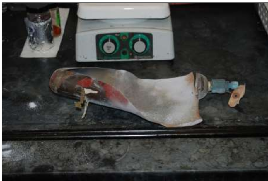
Figure 5.8 – HF Cylinder Incident at Purdue University in 2011
